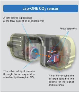
Advanced miniaturization of infrared absorption spectroscopy system
