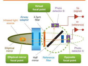
The infrared light is split by a half mirror and concentrated into two photo detectors. Photo detector A at the opposite focal point of the elliptical mirror detects the reference beam. Photo detector B at a virtual focal point 90° from photo detector A detects the signal beam from the half mirror.
