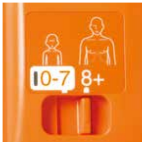
AED-2152K can be used for child by only changing mode switch.
